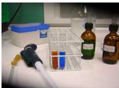
Slika 85: Fehlingov test na glukozo (levo) in saharozo (desno) pred hidrolizo Vir: http://www.scienceinschool.org/2007/issue4/enzymes/ (5.1.2010)
